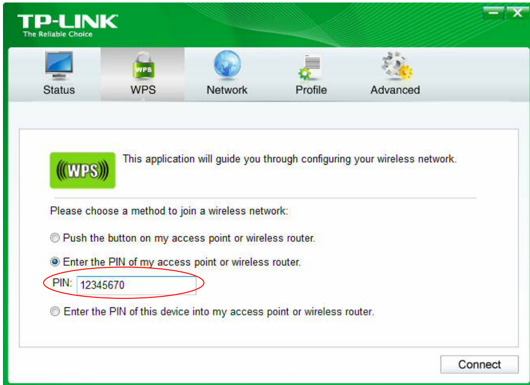
Figure 4-9 The WPS Configuration Screen of Wireless Adapter [Ecran de configuration WPS de l'adaptateur sans fil]
